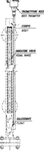
Code : **N** (std employment) : EX (EExi employment) : **HR** (HART<sup>®</sup> protocol) It is available the version for employment in ambient with explosion danger, trough a probe certificated EExia IIC T1-T6. The level trasmitter is also suppliable with HART<sup>®</sup> protocol for employment in ambient with explosion danger. HOW TO ORDER : example : TL. 200.N
