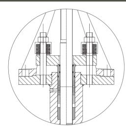
In addition to this device and for oxygen service, Viton O-rings are placed on the gland follower on inner and outer diameters in order to avoid entry of foreign substances within the gate valve body shell. O-rings also contribute to increase stuffing box efficiency. This gland follower is also equipped with a scraper that cleans the stem surface during the valve closing phase.
